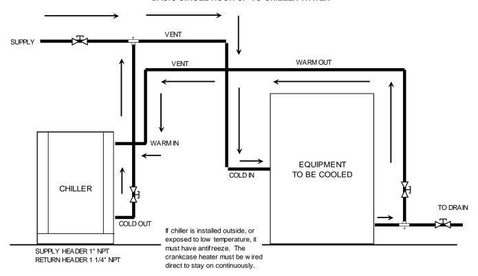
Use any std. w ater pipe. DO NOT plumb w ith smaller size pipe than noted on this print. The bypass line is necessary if units to be cooled have self acting shut-off valves. Water must circulate through chiller at all times for proper operation and temperature control. Place bleeder valve at highest point and fill unit until w ater discharges from bleeder. Close bleeder -- unit is full. Shut off outside w ater supply.
